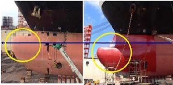
Remodeling of the ship's bulbous bow (Left: Before remodeling) (Right: After remodeling)
